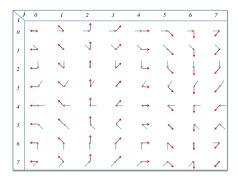
**Fig. 1.** Representation of motion comparisons of patches from three successive frames. For a given pixel and frame, blue arrows show the motion from a patch in the preceding frame and red arrows show the motion to a patch in the succeeding frame.
