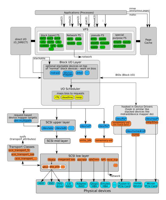
Figure 1.1: The Linux I/O Stack. The figure outlines Linux i/o stack as of kernel version 3.3 *Figure created by Werner Fischer and Georg Schönberger and used under the Creative Commons License.*
