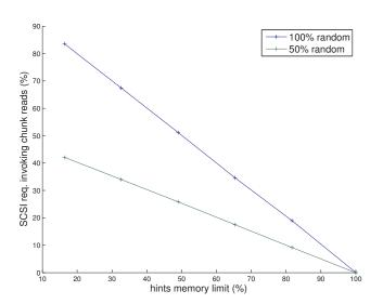
Figure 2.5: The effect of limiting the memory allocated for hints storage on the host-side device driver. The 100% point allows the entire page-level mapping to be stored on the host. The blue line displays the behavior in a purely random workload, and the green line in a workload where only 50% of the requests are random and the rest are sequential.
