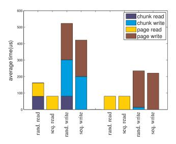
Figure 2.4: The impact of hints when bus transfer times drop to 5ns per byte.
