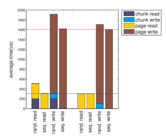
Figure 2.3: The impact of hints on our SSD when flash read and program times are longer (200*u*s and 1.5ms, typical of some 3Xnm MLC devices) but bus transfer times remain the same. The impact on writes becomes smaller, because of the long latency, but the impact on reads becomes larger.
