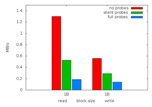
Figure 3.3: The graph shows read/write performance using I/O block of size 1 byte. This small block size emphasizes the overhead introduced by using SystemTap
