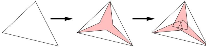
**Figure 15.** Replacing a fat triangle by three canonical triangles.
