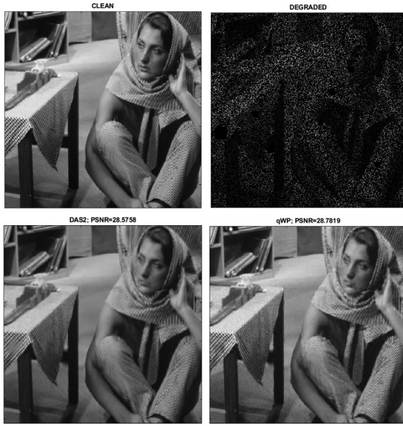
Fig. 4.8. Restoration of “Barbara” image. Left: Top left: clean image. Top right: image degraded by application of modified mask4 (80% of pixels and square patches are missing). Bottom: Restoration by M2 (right), PSNR=28.78 dB, SSIM=0.7312 and by DAS-2 (left), PSNR=28.58 dB, SSIM=0.7471. Right: Image fragments. Columns: First — clean fragments; Second — degraded; Third — restored by DAS-2; Fourth — restored by M2 . Bottom row — gap of size 32 \times 32 , in the rest of rows — gaps of size 16 \times 16 .
