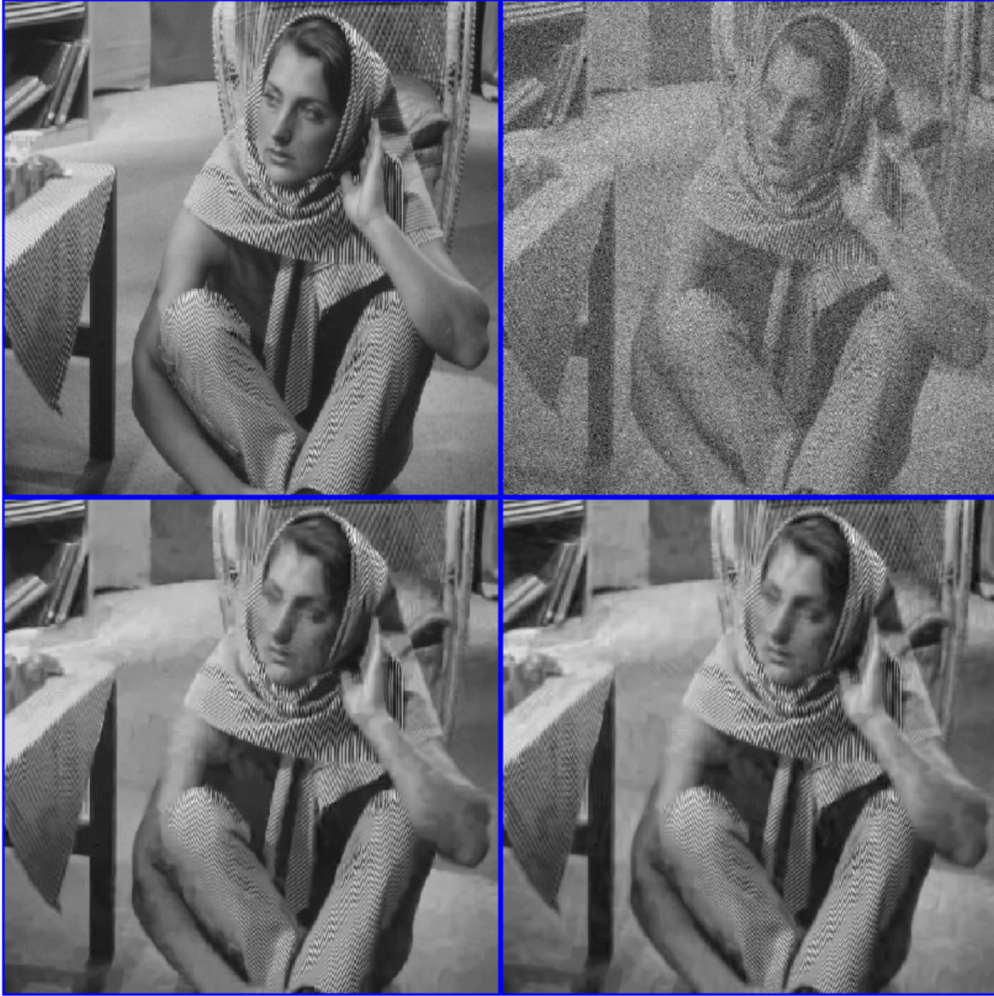
Fig. 7.3. Top left: Original “Barbara” image. Top right: Image corrupted by noise with \sigma=40 dB, PSNR=16.09 dB. Bottom right: The hybrid-restored image \mathbf{X}_h , PSNR=28.55 dB. Bottom left: BM3D restored image \mathbf{X}_{bm} , PSNR=28.19 dB.
