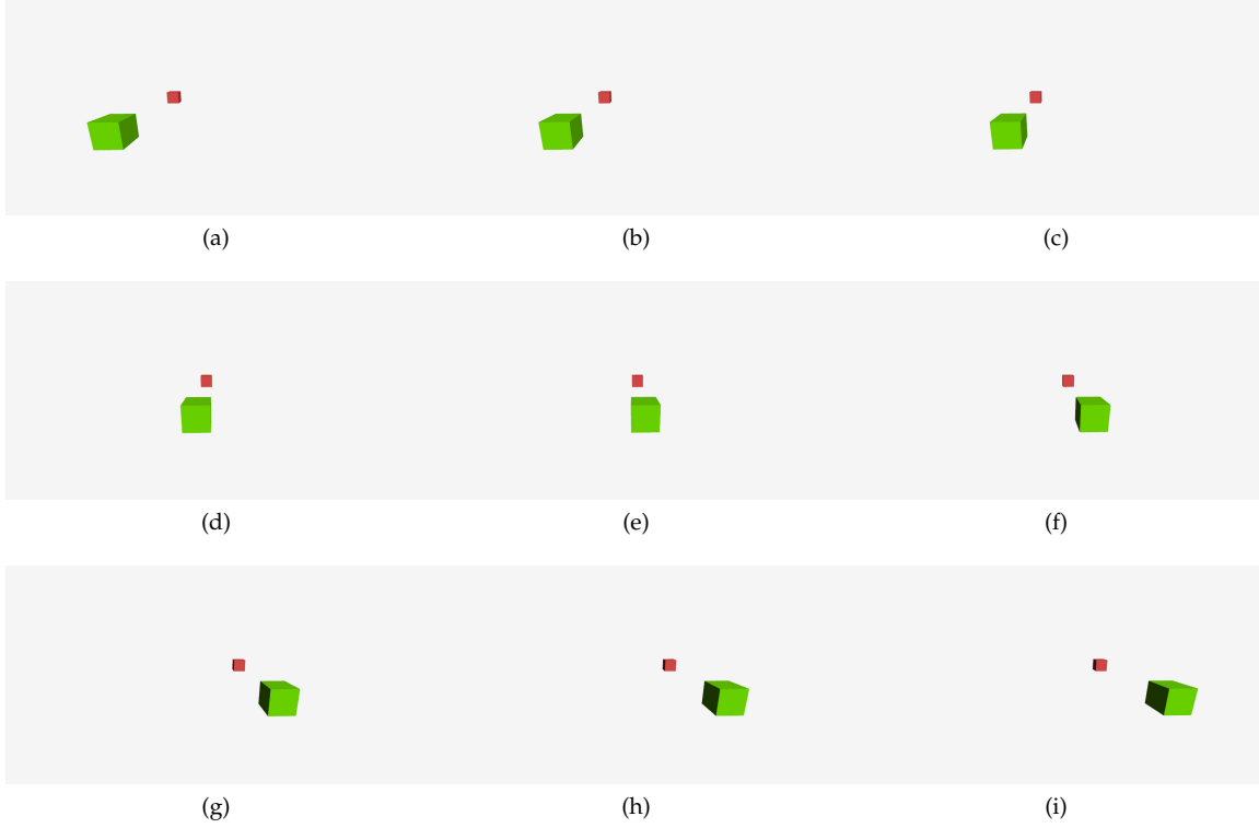
Fig. 3.3: Images taken at constant time intervals from a camera moving at constant speed from right to left. The green box, which is closer to the camera, appears to be moving faster than the distant red box.
