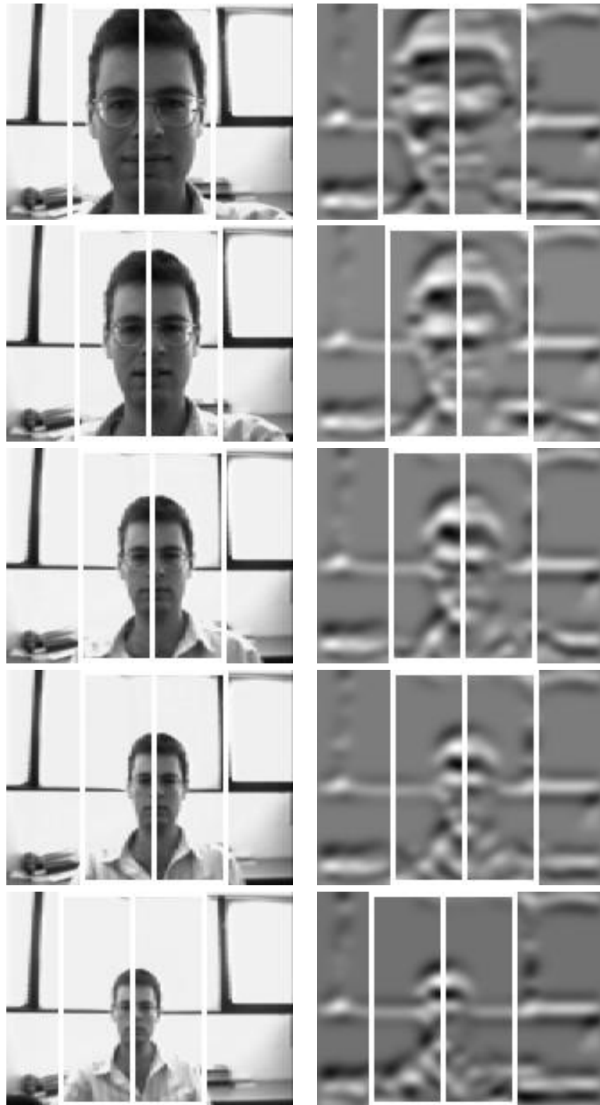
Figure 5: Robustness to scale. Several scales of the face. The Y-Arg image strongly reacts to the eyes and hair regions, regardless of the scale. Largest face is about 6 times larger than smallest face. Detection by mirrored auto-correlation is marked.
