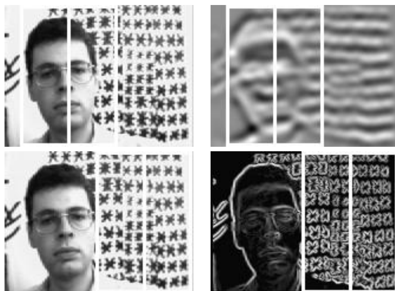
Figure 10: A texture of asterisks. Facial edges look negligible near texture edges. In the Y-Arg map, facial regions attain higher values than textural areas.
