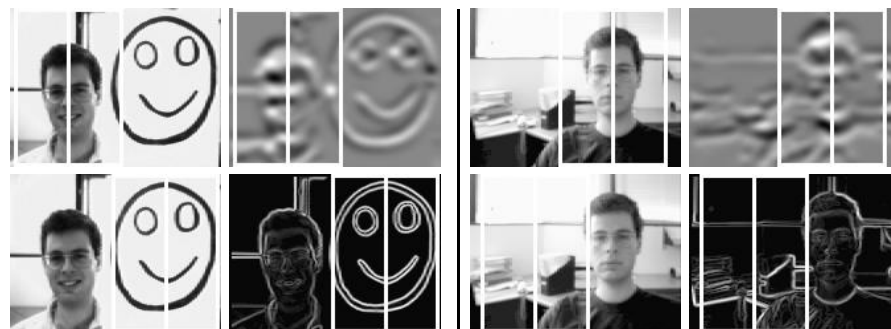
(a) A face vs. smiley. Edge-based methods locate the larger object, which is the flat smiley. Y-Phase detects the three dimensional face, although it is smaller.
