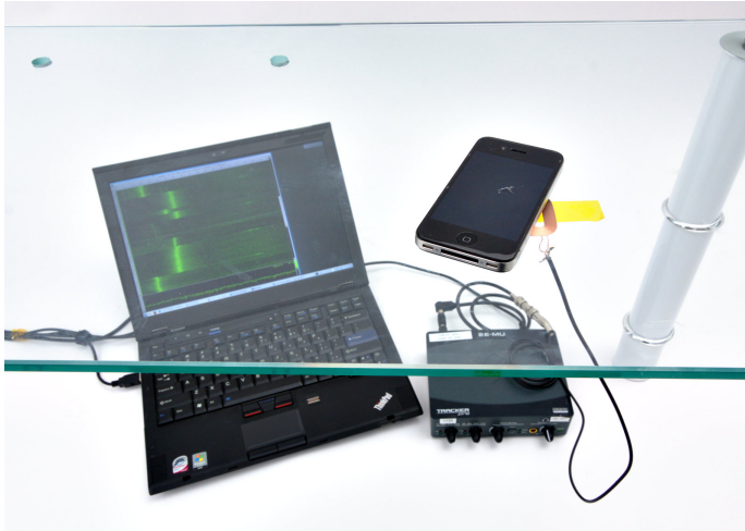
(a) Top view. The target (top right) is measured by the improvised probe (taped to the underside of a glass table). The signal is captured by a Tracker Pre sound card connected to a laptop (under the table).
