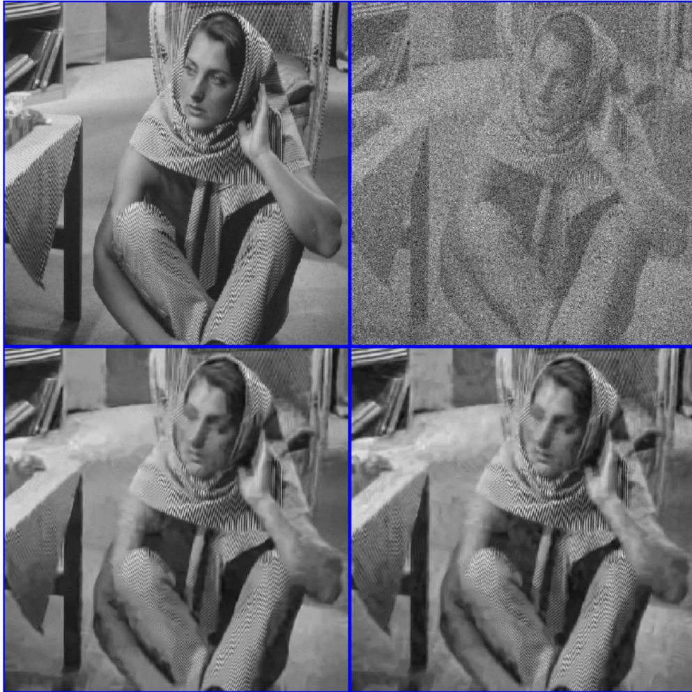
Fig. 7.5. Top left: Original “Barbara” image. Top right: Image corrupted by noise with \sigma=60 dB, PSNR=12.57 dB. Bottom right: The qWPT–BM3D-restored image \mathbf{X}_h , PSNR=26.51 dB. Bottom left: BM3D-restored image \mathbf{X}_{nd} , PSNR=26.34 dB.
