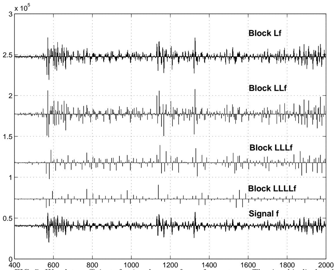
FIG. 7. Wavelet coefficients for 4 scales transform of a sea trace. The signal is displayed in the bottom plot.
