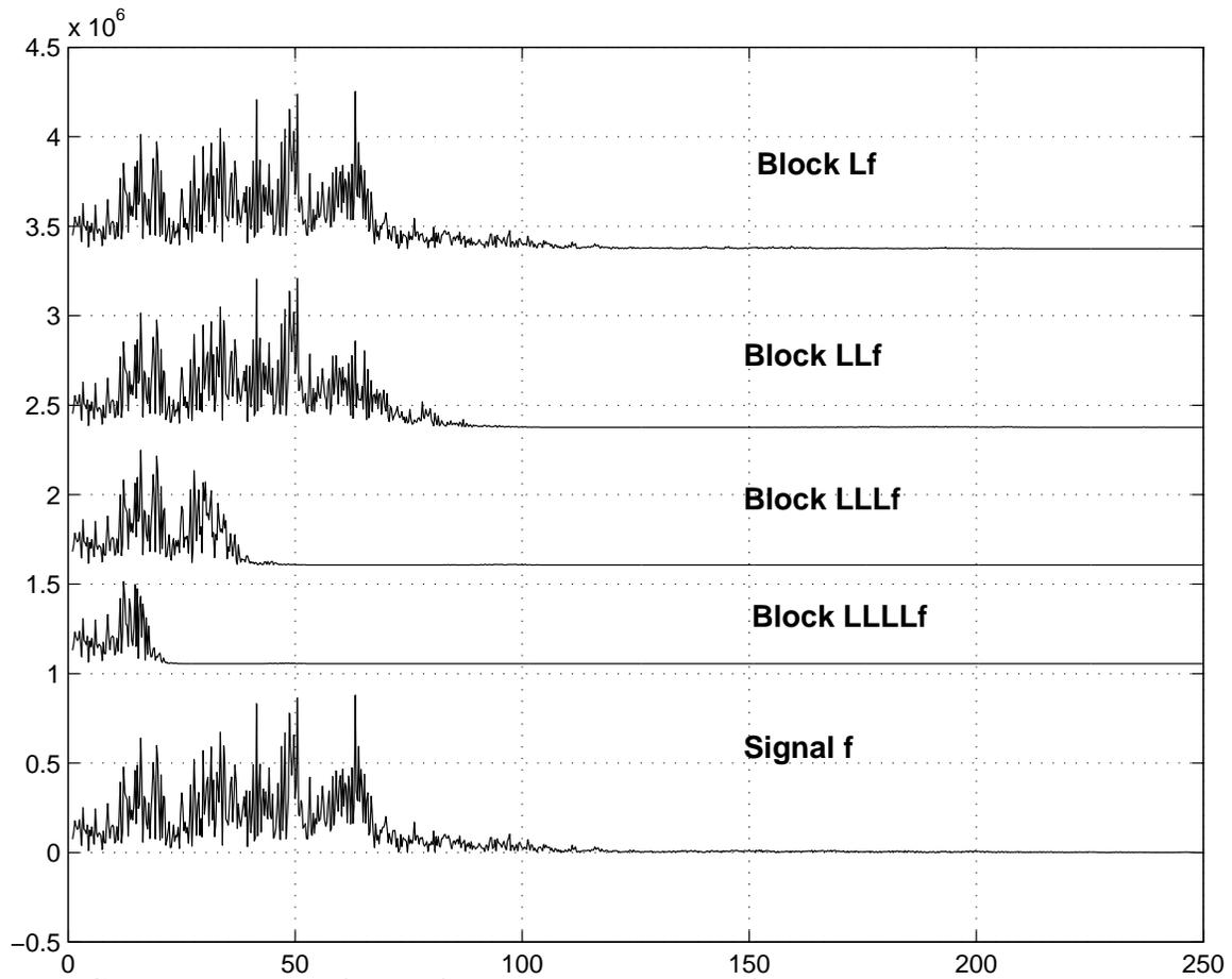
FIG. 9. Fourier transforms of the reconstructed low-frequency blocks displayed in Figure 8. The spectrum of the signal is displayed in the bottom plot.
