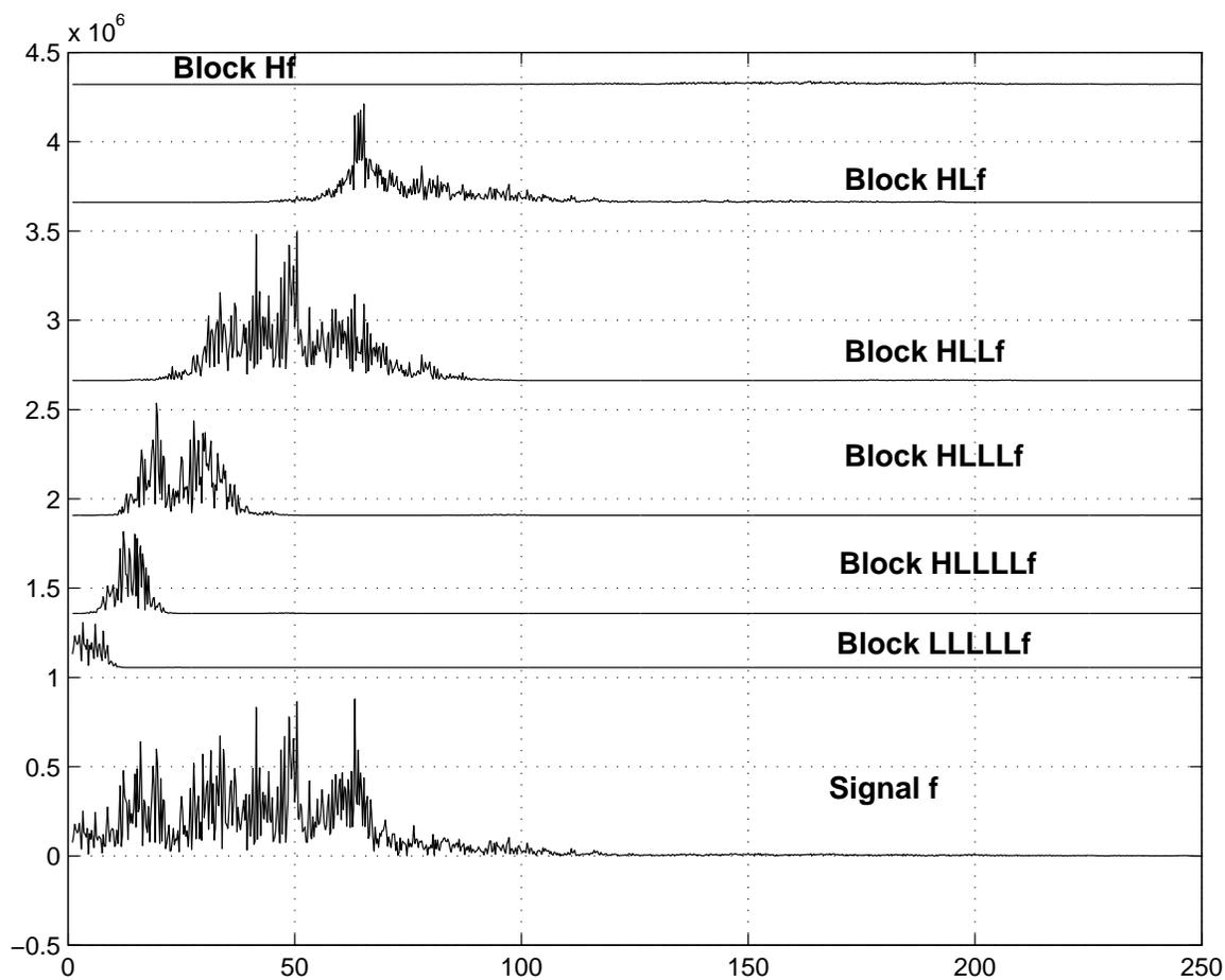
FIG. 3. Fourier spectra of the scale-wise reconstruction of the seismic signal from 5 scales. The spectrum of the signal is displayed in the bottom plot.
