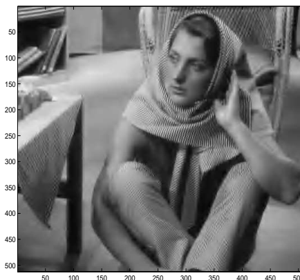
Figure 1.14. Left: “barbara”: Reconstructed from 40:1 compression. The B7/9 filter was applied: PSNR=25.78. Right: T_2^1 transform: PSNR=25.50.
