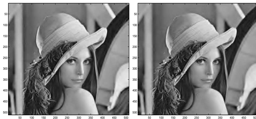
Figure 1.12. Left: “Lena”: Reconstructed from 40:1 compression, the B7/9 filter was applied: PSNR=31.42. Right: T_1^2 transform: PSNR=31.47.
