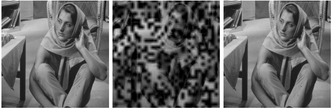
Figure 6: Results from the application of the antisymmetric tight framelet transform. Left: corrupted image with 60% erased coefficients. Right: recovered image. PSNR = 32.24.
