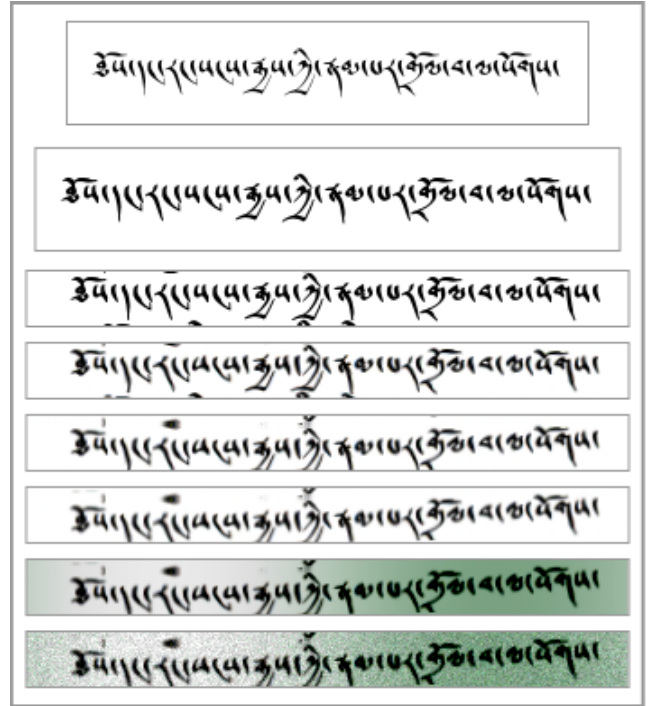
Fig. 1. Illustration of the text augmentation procedure. The first two images are renderings of text using different font sizes, stretch, weight and spacing; the 3rd is the text after rendering it together with adjacent lines and performing line segmentation; 4th is the result of performing elastic deformation augmentation on the image; 5th is after sinusoidal displacement; 6th is after rotation; 7th is after intensity gradient noise; 8th is after adding white Gaussian noise.
