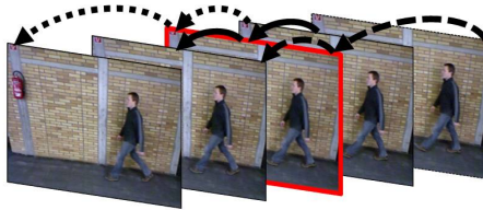
Fig. 4. Visualization of the Temporal MIP extension. Standard MIP encodes three successive frames, t - 1 , t and t + 1 (solid arrows). Temporal MIP additionally encodes frames t - 1 , t and t + 2 (dotted arrows), and frames t - 1 , t , and t + 2 (dashed arrows). Frame t is emphasized in red.
