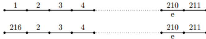
Figure 1: Example for two different rankings that result in long dependency chains. Note that in both cases in order to determine whether the edge marked e belongs to M the algorithm must recursively check all edges preceding it in the ranking
