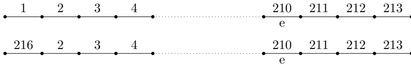
Figure 1: Example for two different rankings that result in long dependency chains. Note that in both cases in order to determine whether the edge marked e belongs to \mathcal{M} the algorithm must recursively check all edges preceding it in the ranking
