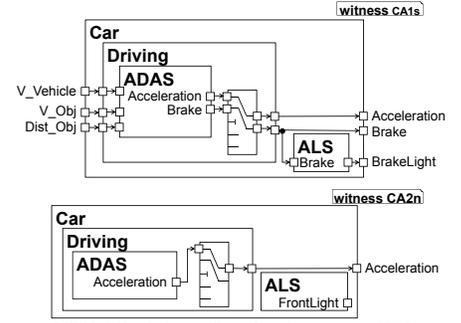
C&C Model is missing an effector from the component ADAS to the component ALS (from port Acceleration to port FrontLight)
