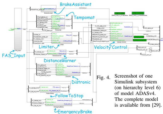
Fig. 4. Screenshot of one Simulink subsystem (on hierarchy level 6) of model ADASv4. The complete model is available from [29].
