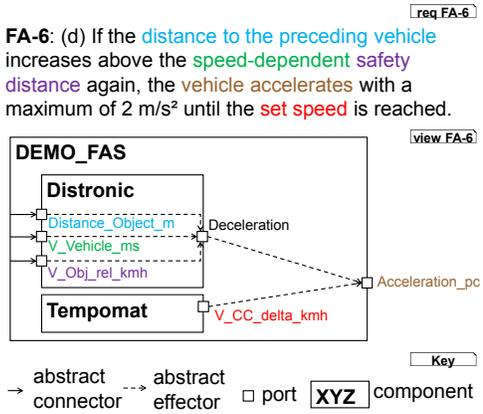
Fig. 5. Requirement FA-6 of unit Distronic of ADASv4 (top) and the view created for the requirement by the domain experts (bottom)
