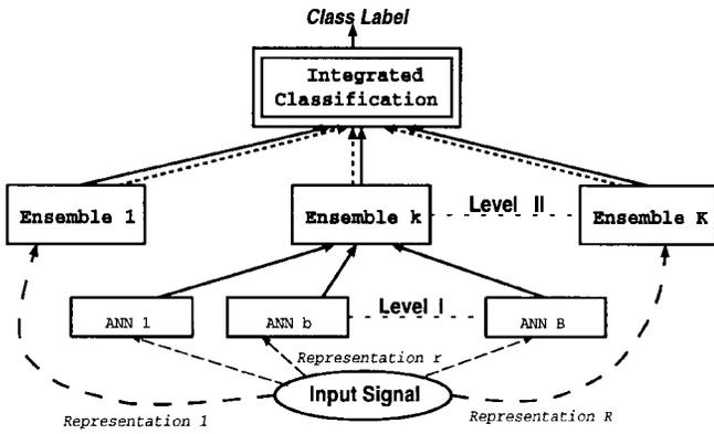
Fig. 2. Integrated classification machine. Several representations of the waveform are fed into different ensembles, then integrated to produce the final classification. (In level II, the regular arrows are the ensembles' prediction values, and the dashed arrows are the attached confidence values).
