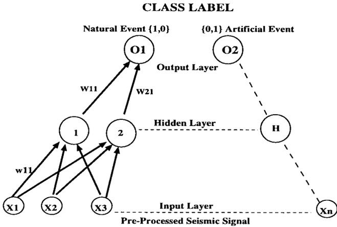
Fig. 1. Feed-forward neural network with input dimensionality  $N$  and one hidden layer with  $H$  units and two output units as used for classification in the ICM.
