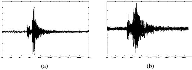
Fig. 3. (a) Natural earthquake event. (b) Artificial explosion event. The horizontal axis is recording time in seconds (The sampling rate is  $50 H_z$ ).
