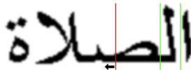
Figure 3. A word consisting of 3 subwords processed by SOCR (green lines are segmentation points; red line is the end of the sliding window).
