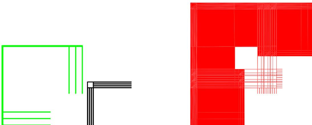
Figure 1.2:  $P$  and  $Q$  are non-convex polygons with  $m$  and  $n$  vertices respectively. The complexity of  $P \oplus Q$  is  $\Theta(m^2n^2)$ . This is the worst case scenario. (Computed with Eyal Flato Minkowski Sum package [9].)
