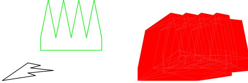
Figure 2.2:  $P$  and  $Q$  are non-convex polygons with  $m$  and  $n$  vertices respectively,  $P$  is  $x$ -monotone and  $Q$  is  $y$ -monotone. The complexity of  $P \oplus Q$  is  $\Theta(nm\alpha(\min(n, m)))$  and the boundary can be presented as the concatenation of two  $x$ -monotone and two  $y$ -monotone connected polygonal chains. (Computed with Eyal Flato Minkowski Sum package [9].)
