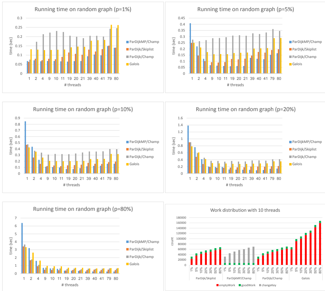
■ Figure 7 SSSP algorithms with different priority queues: Run time (lower is better) and work distribution.
