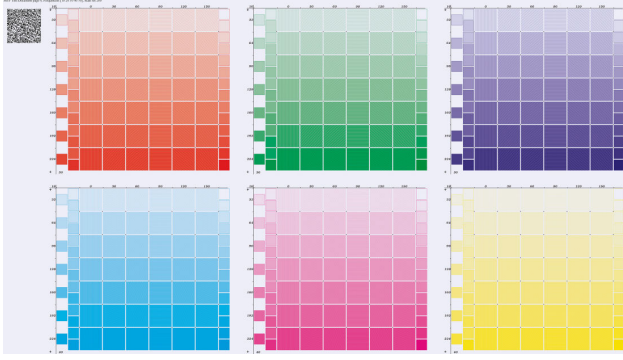
Figure 3. Patches are set in test grids varying over angle and luminance, and then on pages grouped by frequency.
