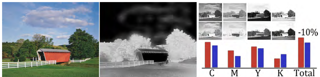
Figure 1: In preparing an image for print (left), we reduce ink usage by detecting areas which are active (middle, brighter is more active) i.e. contain detailed textures, edges and structure. In these areas we are able to use less cyan, magenta and yellow ink while increasing use of black ink. We are able to reduce ink usage (right) by up to 25% (10% in this example) without degradation in printed image quality.
