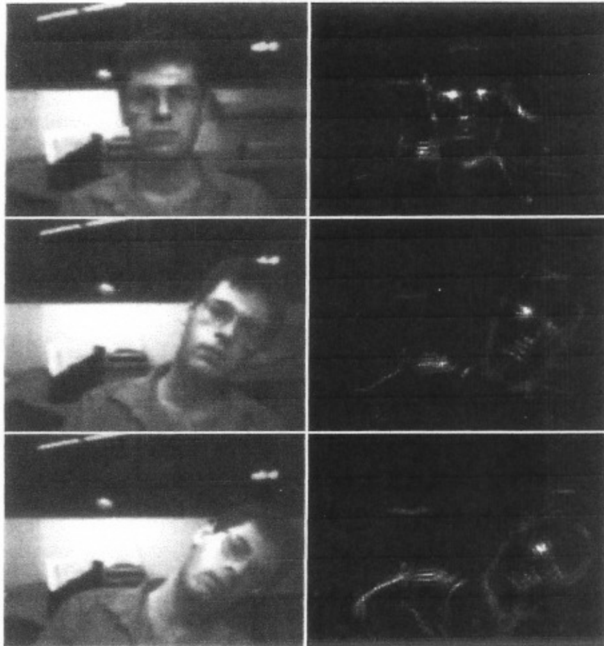
FIG. 8. Detection of eyes in tilted images. Face images of various tilt angles (left), and the response of the symmetry transform (right). The same parameters are used in all three images.
