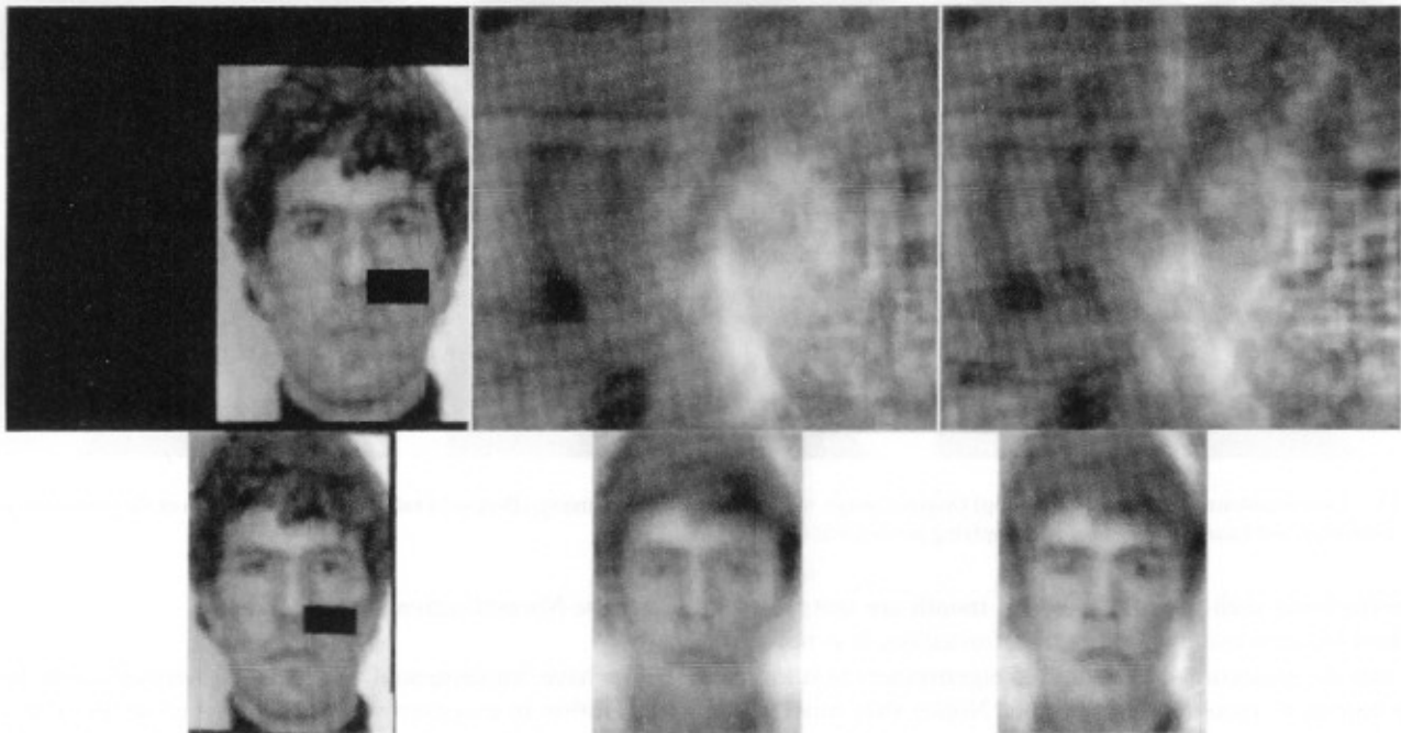
FIG. 15. Projection of a new face on a principle component space. (Top) A new image (left), projection on 25 eigenvectors (center), and on 40 eigenvectors (right). (Bottom) The same as the top but applied to normalized images by the location of the eyes and the mouth.
