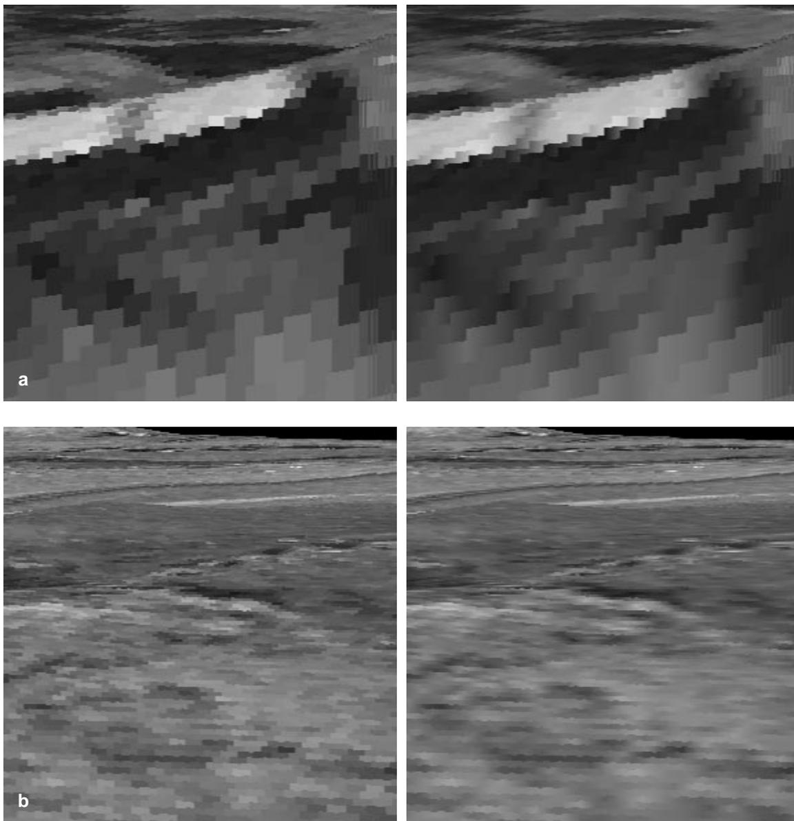
**Fig. 5.** Linear interpolation versus point sampling. Images generated by point sampling are on the left side, while images created by linear interpolation are on the right side: **a** the camera is very close to the voxels, emphasizing the smoothness of the filtered image; **b** the camera is a little farther away, but still close enough to emphasize the effect of the filtering
