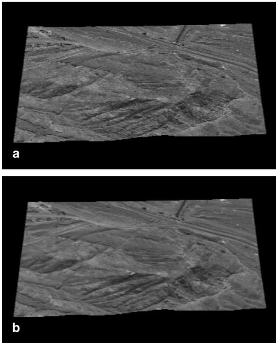
Fig. 1. The quality of an output image using: **a** point sampling; **b** supersampling
