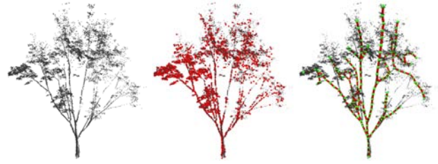
(a) Raw scan. (b) Initial samples. (c) Skeleton.
