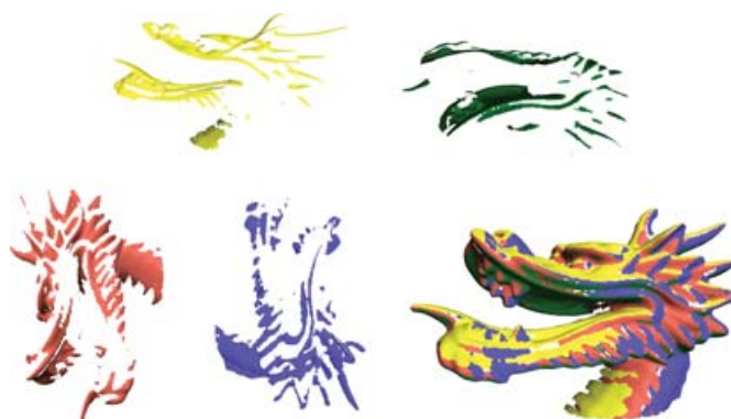
Fig. 22. Registration of four synthetic scans. The surface of each scan has normals enclosed in a normal cone. Matches of overlapping areas were found using our method.
