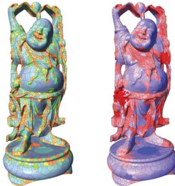
Fig. 8. The left image shows the local surface descriptors colored by the curvatures. In the image on the right, the saliency grades are visualized on a scale from blue to red. The patches are colored according to the saliency grade of the salient feature that contains them.
