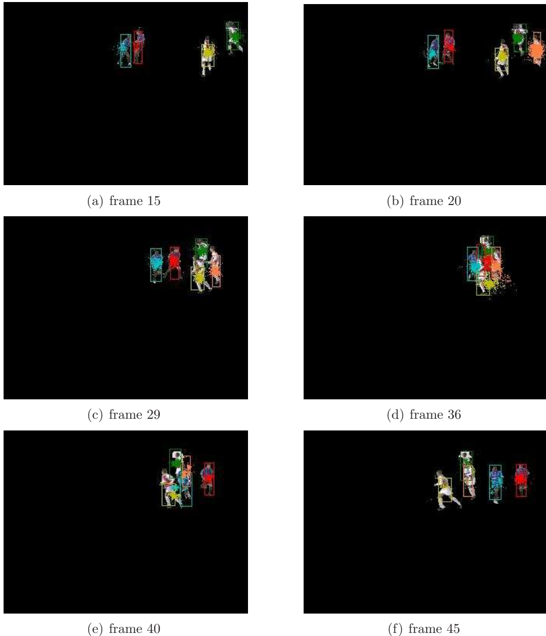
Figure 7.6: An example of tracking soccer players where occlusion between five players is present.
