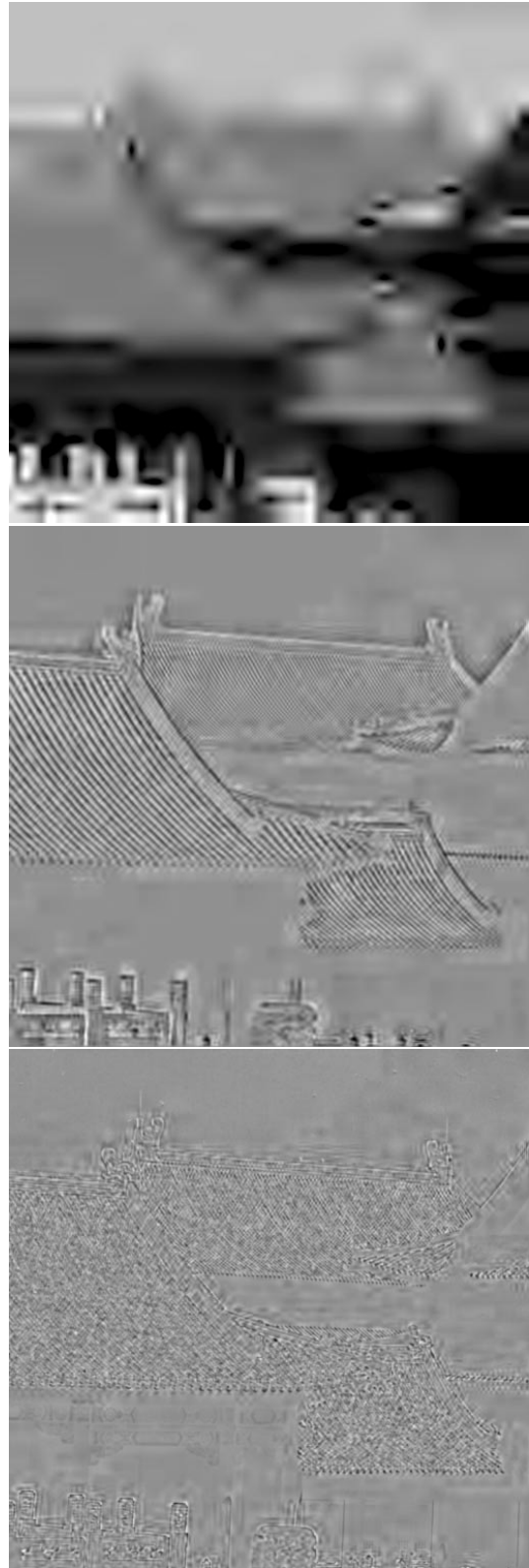
Fig. 4. The first layer, \hat{R}^0 , is the decoded image after a wavelet compression by a factor 750 of the original image, and this layer constitutes the first residual R^1 . Center : the second layer, \hat{R}^1 , is reconstructed after a compression by a factor 70 of the first residual R^1 using a local cosine basis. Bottom : the second residual R^2 is the difference between the first residual R^1 and the second layer \hat{R}^1 .
