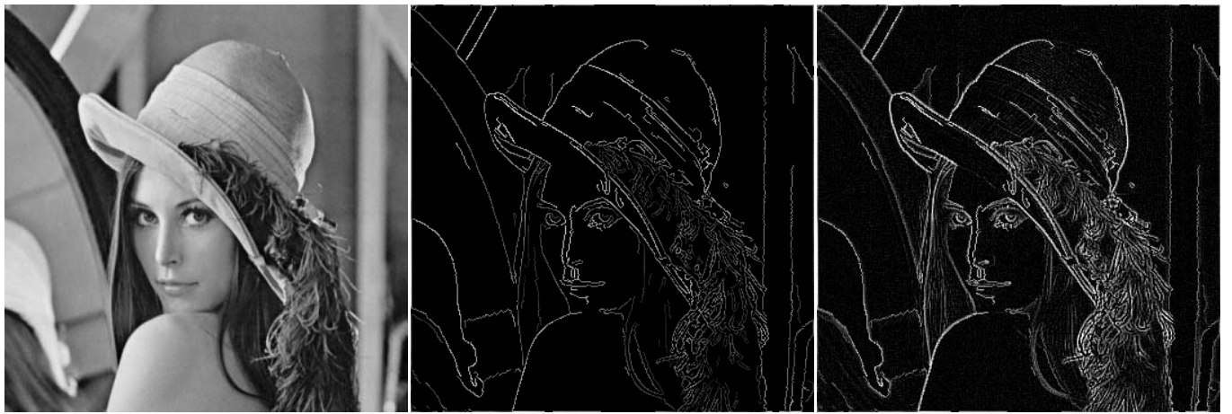
Figure 6.7: Left: Original image with the additional of 5% uniform noise. Middle: The output from the application of the Canny edge detection on the left image. Right: The output from a Canny edge detector + artificial dissipation on the left image.
