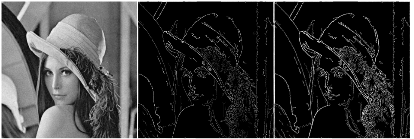
Figure 6.9: Left: Original image with the additional of 15% uniform noise. Middle: The output from the application of the Canny edge detection on the left image. Right: The output from a Canny edge detector + artificial dissipation on the left image.
