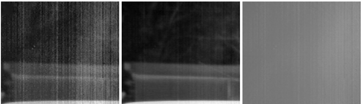
Figure 22: After 31 iterations. Left: non-uniform, center: corrected, right: residual.
