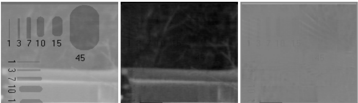
Figure 36: After 31 iterations. Left: non-uniform, center: corrected, right: residual.
