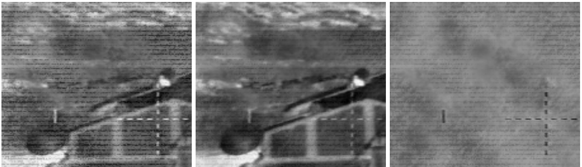
Figure 28: After 7 iterations. Left: non-uniform, center: corrected, right: residual.
