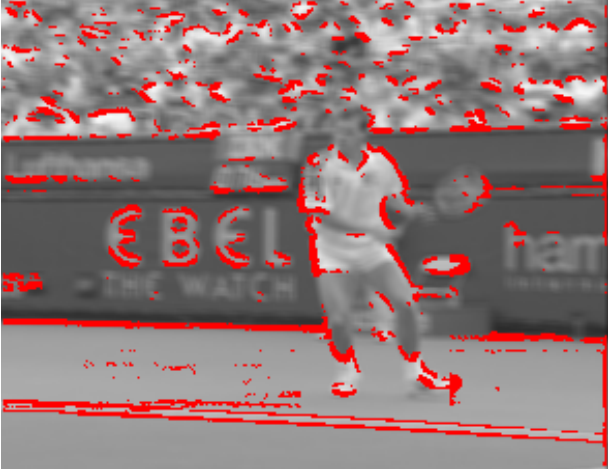
Fig. 2. An example of the locations of the subset of pixels used for the global motion computation. The pixel set is superimposed on the first frame of the Stefan video sequence.
