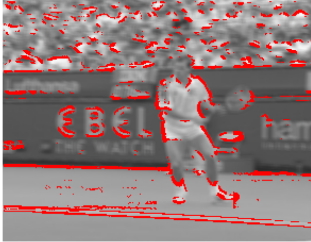
Figure 2: An example of the locations of the subset of pixels used for the global motion computation. The pixel set is superimposed on the first frame of the Stefan video sequence.
