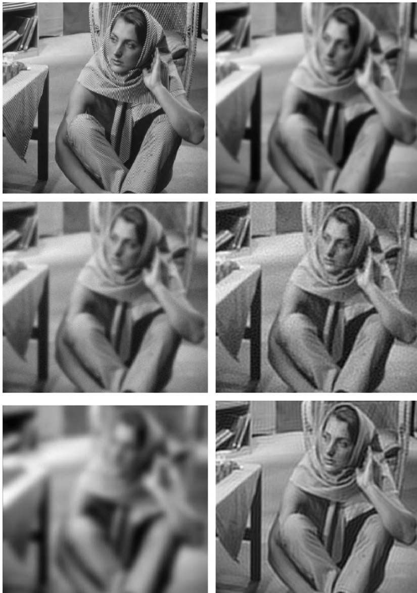
Fig. 3. Barbara. Top left: the original f(x, y) = u(x, y, 0) . Top right: the solution u(x, y, 5) , PSNR = 22.96. Center left: solution u(x, y, 5) corrupted by Gaussian noise, PSNR = 22.63. Center right: inversion by the spline of fourth order PSNR = 23.53. Bottom left: solution u(x, y, 40) , PSNR = 20.31. Bottom right: inversion by the spline of eighth order S_\rho^{8.8}(x, y) , PSNR = 23.69.
