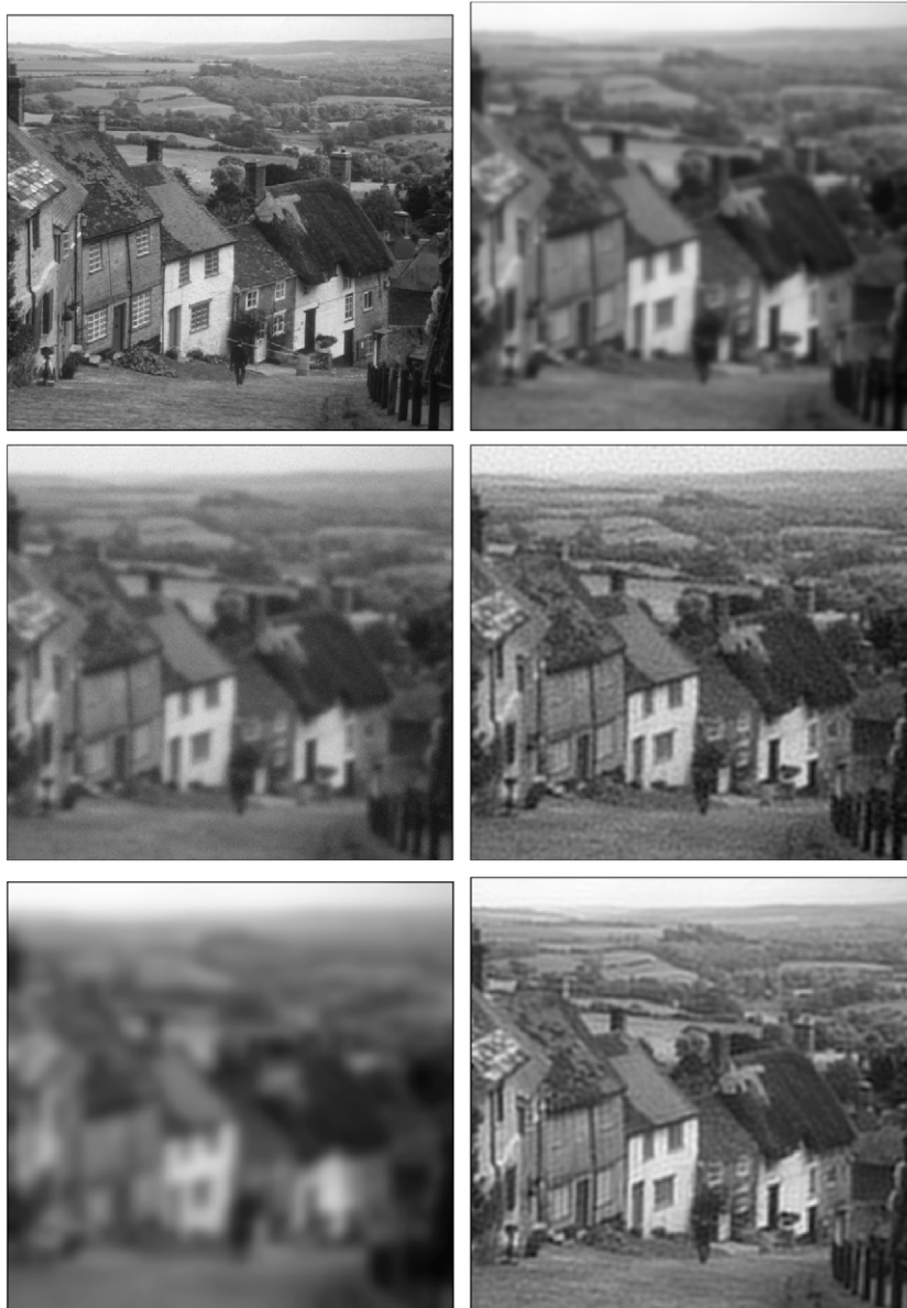
Fig. 4. Goldhill. Top left: original f(x, y) . Top right: convolution with g_{\sigma}(x, y) , \sigma = 3 , PSNR = 26.8. Center left: convolution with g_3(x, y) corrupted by Gaussian noise, PSNR = 25.21. Center right: inversion by spline of sixth order S_{0,0.15}^{6,6} , PSNR = 27. Bottom left: blurred image, PSNR = 22.53. Bottom right: inversion by spline of third order S_{\rho}^{3,3} , PSNR = 27.74.
