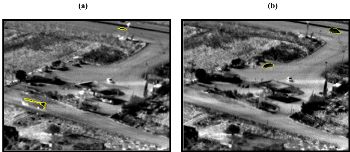
Figure 13: The outcome from the change detection algorithm after comparing I_1 (image a) relative to I_2 (image b) and I_2 relative to I_1 from the images in Figure 10. Each 'object of change' is surrounded by a yellow contour.
