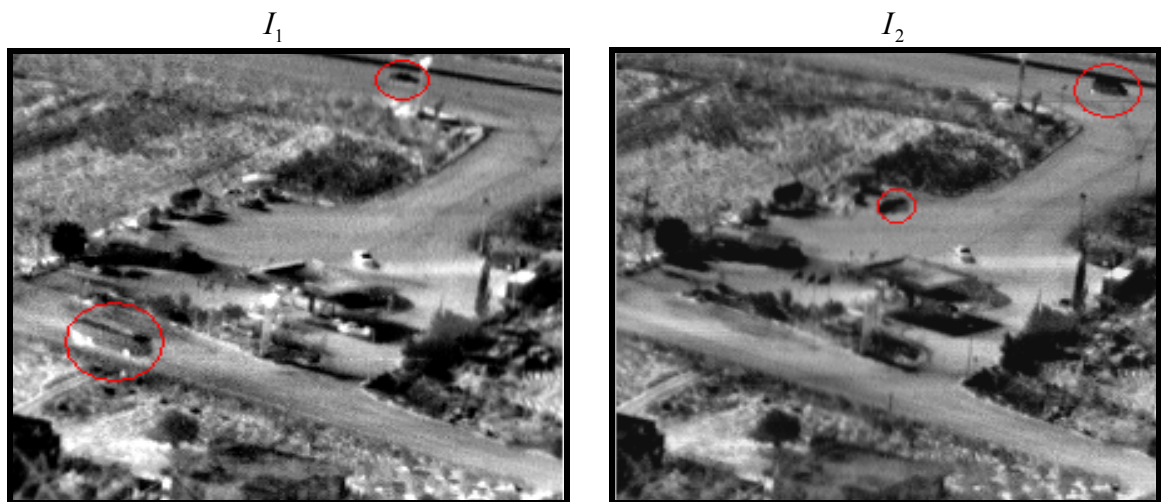
Figure 10: Pair of registered gray levels input images that were captured with a lag of two hours between them. Each image contains two different objects which do not exist in the other.
