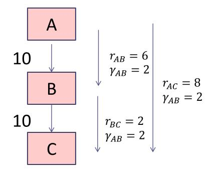
Continue increasing flows equally. When AB and AC get each 5, edge (A,B) is saturated.
