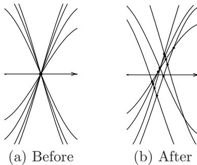
Figure 8: Arcs at the vicinity of a touching point: the effect of displacing polygon vertices
