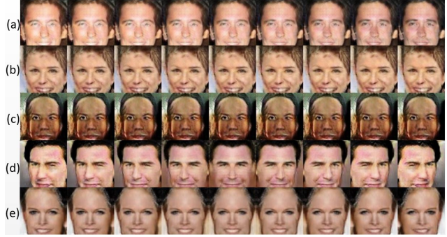
Figure 9: Series of images generated by various GAN methods, trying to obtain a mirroring effect between images on the left and right side of each series. (a) DC-GAN. The first 5 elements of the 100D vector z change, but this has little effect on the output image. (b) DC-GAN with a soft symmetric loss term, using the z' encoding of symmetry. (c) DC-GAN with a strong symmetric loss term and using the z' encoding of symmetry. (d) Symmetric-GAN using the z' architecture. (e) Symmetric-GAN using the flip architecture.
