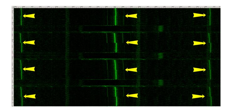
Figure 4: Chassis measurement (1.7 sec, 1.9–2.6 MHz) of four GnuPG RSA signatures executed on a Lenovo 3000 N200. The transitions between p and q are marked with yellow arrows.
