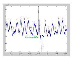
Figure 9: Frequency demodulation of a segment of the leakage signal obtained during a decryption operation using a randomly generated 4096-bit RSA key. Note the correlation between the signal and the secret key bits.
