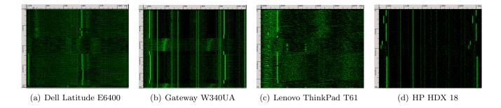
Figure 2: Chassis measurements of various target computers performing MUL, HLT and MEM in this order. Note that the three operations can be distinguished on all machines.
