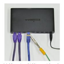
(a) Measuring shield potential at the far side of an Ethernet cable (probed at the Ethernet switch).
