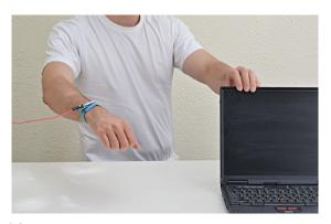
(b) Adaptive "human touch" attack by bare hand. The wristband is connected to the probe wire.
