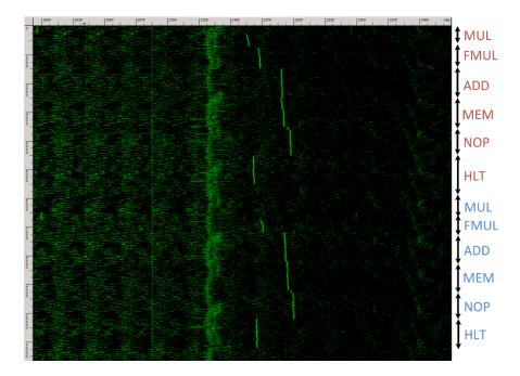
Figure 3: Frequency spectrogram  $(1.1 \, \text{sec}, \, 2\text{-}2.3 \, \text{MHz})$  of a recording of different CPU operations obtained while measuring the attacker's body potential while touching an exposed part of the chassis of a Lenovo 3000 N200 laptop.
