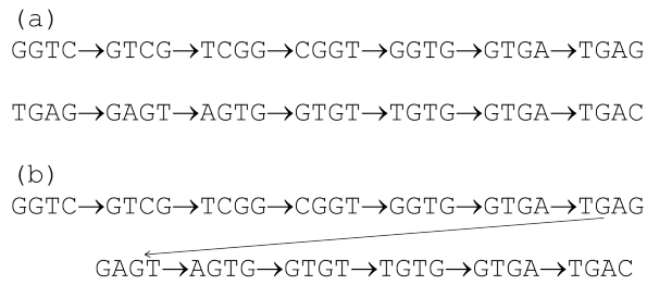
Figure 12.12: The two reads in (a) are converted to paths in the graph, and the common vertex TGAG is identified. Then, we can combine these two paths into (b).
