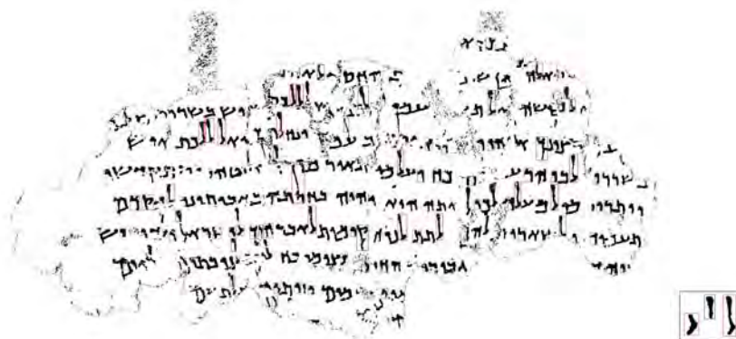
Figure 4.5: Character and partial character matching results of the Hebrew letter lamed. The legend shows the query letters used. The red frames are the keypoints matched to the whole letter, and the blue and magenta frames are the matches of the upper and lower parts, respectively.
